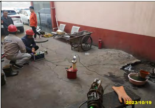
A photograph showing several workers in a workshop setting. One worker in the foreground is kneeling and testing a pair of orange insulation gloves using a specialized device. Other workers are visible in the background, some standing and some working. The floor is concrete, and there are various tools and equipment scattered around. A date stamp '2023/10/19' is visible in the bottom right corner of the image. |
